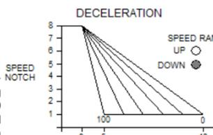
**DECELERATION** The LCC allows the rate of engine speed deceleration to be set. A rate as long as 40 sec. from rated speed to idle is possible. 0 = slowest deceleration. The engine and its load inertia will limit the maximum deceleration rate. In this case, the closed throttle deceleration will be the fastest possible deceleration.
