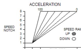
**ACCELERATION** The rate of engine speed acceleration when changing notch settings can be set with this control. The rate as long as 40 sec. or as short as a few seconds from idle to rated speed can be set. 0 = Slowest acceleration.
