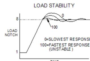
**LOAD STABILITY** The LOAD STABILITY is a time rate adjustment that allows optimization of the load control loop. CCW adjustment compensated for a slow surging of the load. The most stable position is 0 but it also results in the slowest load response.
