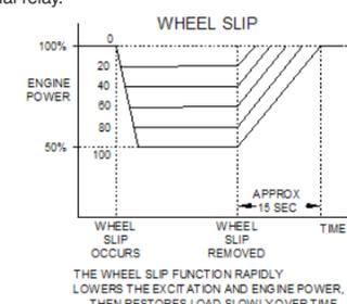
**WHEEL SLIP #2** When wheel slip contact #2 is closed, the field excitation is immediately removed.
