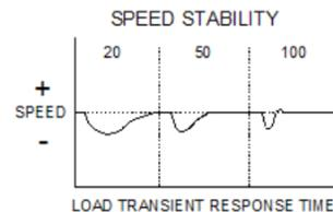
**DROOP** Clockwise adjustment of the droop control will add speed droop to the speed control loop. 0 = Isochronous. 100 = Maximum Droop (about 5%). Droop is proportional to the actuator current change. A small amount of droop can be added to ensure optimal stability at low speeds without interfering with the control system's performance capabilities.
