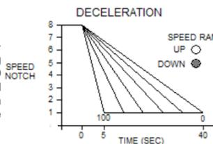
**SPEED NOTCH ADJUSTMENTS 1 - 8** Each notch position has a standard limited range of adjustment. This is usually wide enough to allow for normal variations in the operating speed at each notch. See the specifications for the ranges.
