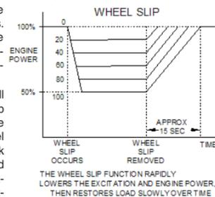
**WHEEL SLIP #2** When wheel slip contact #2 is closed, the field excitation is immediately removed.
