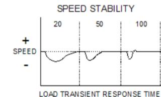
**STABILITY** Clockwise adjustment shortens the time response of the governor. A 25 - 1 range is provided. The longest time constant and the most stable position is the 0 setting.
