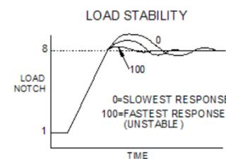
**LOAD STABILITY** The LOAD STABILITY is a time rate adjustment that allows optimization of the load control loop. CCW adjustment compensated for a slow surging of the load. The most stable position is 0 but it also results in the slowest load response.
