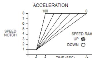
**ACCELERATION** The rate of engine speed acceleration when changing notch settings can be set with this control. The rate as long as 40 sec. or as short as a few seconds from Idle to rated speed can be set. 0 = Slowest acceleration.
