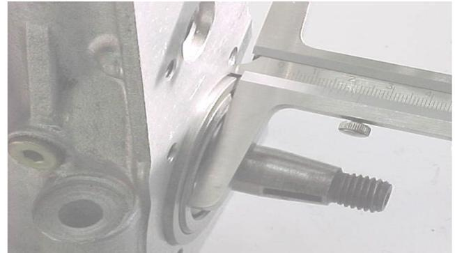
Record this depth as dimension "A". This will be used to determine the required thickness of the clearance shims.
