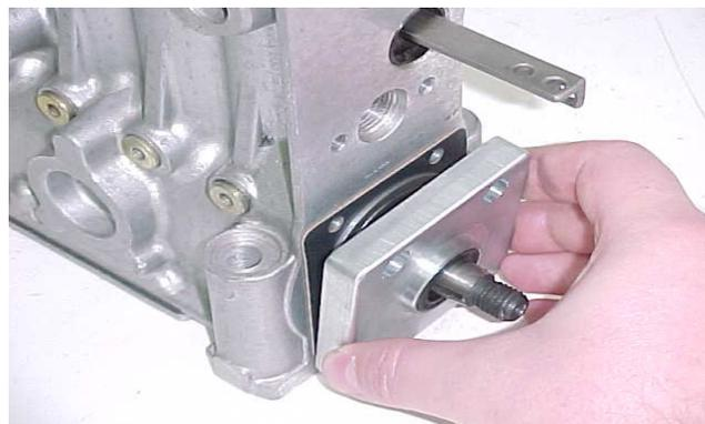
When installing the retainer plate assembly avoid the shaft seal coming into contact with the camshaft keyway channel by carefully pushing the plate away from the keyway, and then sliding the retainer plate into position.
