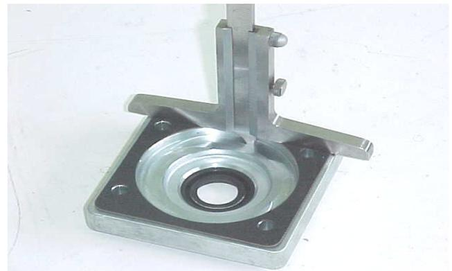
Record this depth as dimension "B". The dimension in the bearing retainer plate will be larger than the bearing dimension "A" on the fuel pump.
