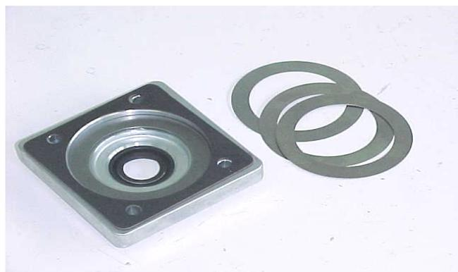
Hold the shims in the plate with the application of a small amount of grease.
