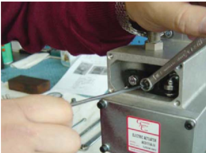
Max Fuel Adjustment, Setting Either Rack Travel or Fuel Flow On a Test bench
