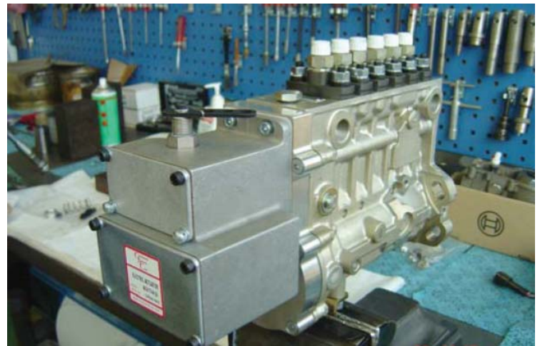
Fig.6. MOTORPAL Pump w/ KT153 and Actuator Installed
