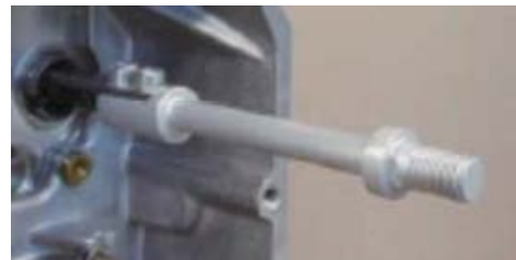
FIGURE 4 RACK LINE EXTENSION
