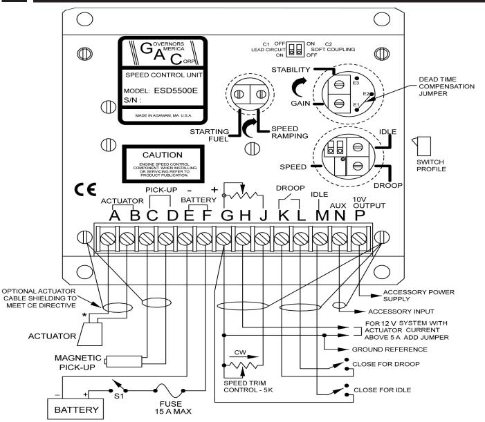
\*SEE SPECIFIC ACTUATOR PUBLICATION FOR WIRING DETAILS BASED ON BATTERY VOLTAGE
