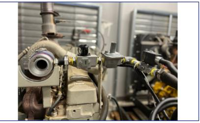
GAC's dual-fuel conversion controls the flow of gaseous fuel and does not affect the diesel fuel system. As load increases, a load signal is used to determine the required increase in power. The gaseous fuel enters the inlet air stream through a shutoff solenoid, gas pressure regulator, mixer, and fuel control valve.
