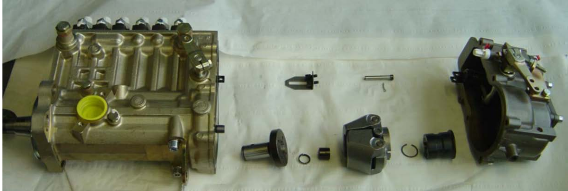
FIGURE 2 DISASSEMBLED MECHANICAL GOVERNOR ON MOTORPAL PPXM PUMP
